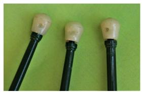
Littletown lamp heads with what appear to be casting flaws. Note the gaps between the head and the base.
